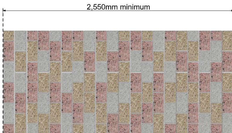
Randomised grey, pink and buff 120mm x 220mm granite sett paving to identify and give warning of pedestrian intersections
